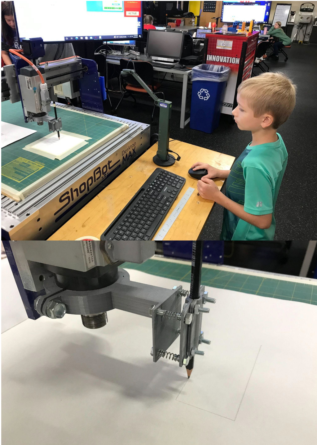
Here a participant uses a pencil tool to draw with a CNC machine.
